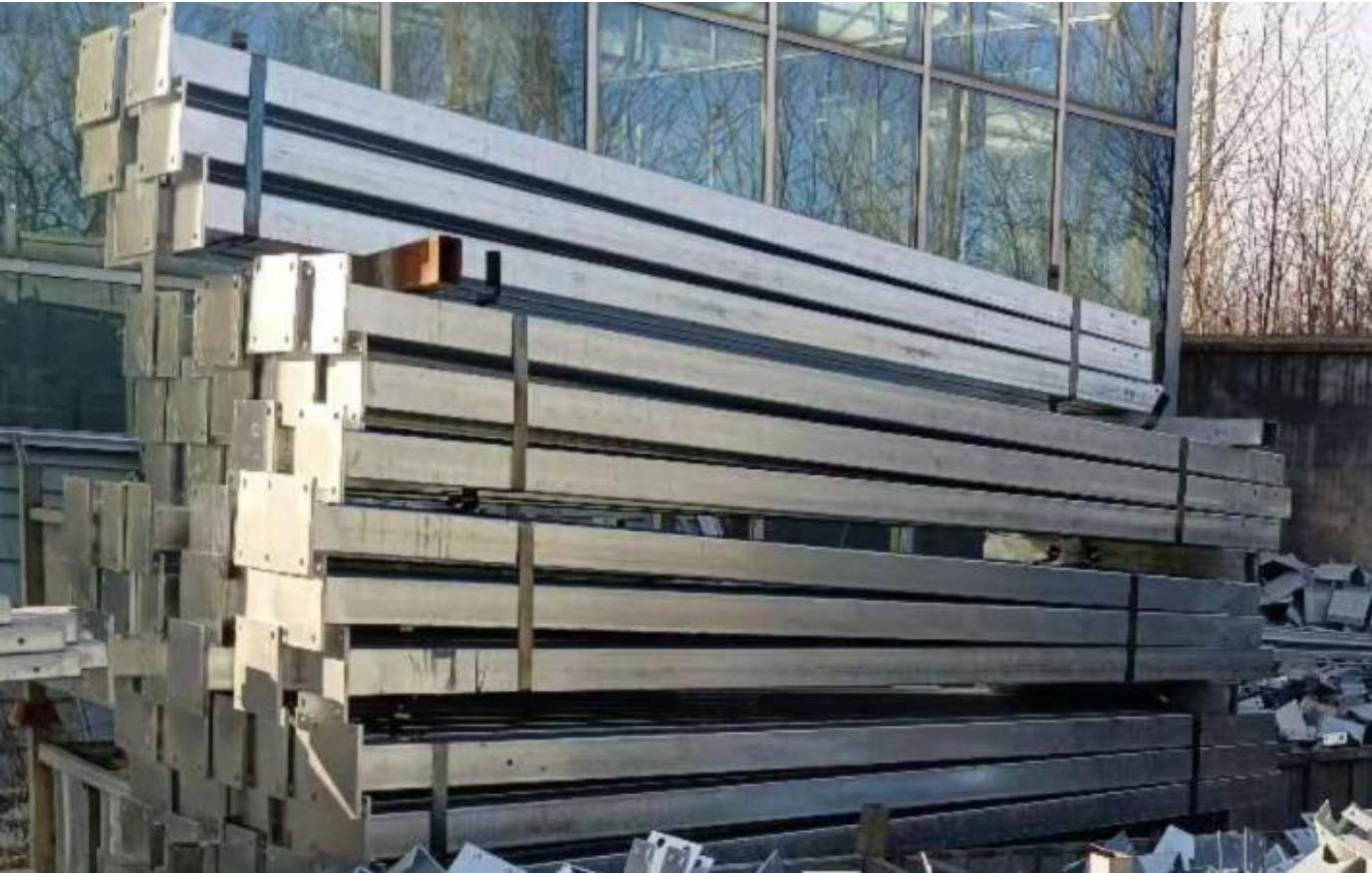
The column welded with bottom plate
